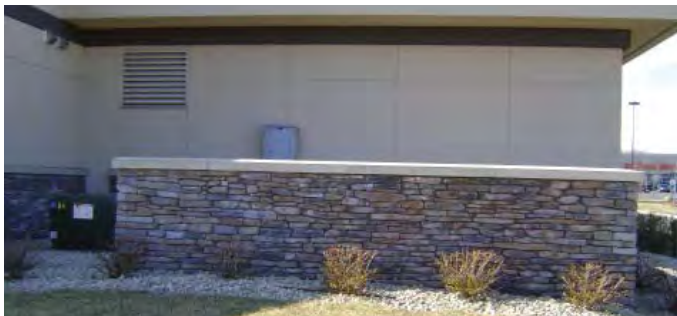
Architectural materials and landscaping help to minimize views of utility cabinets and equipment, while providing limited access for maintenance and use
