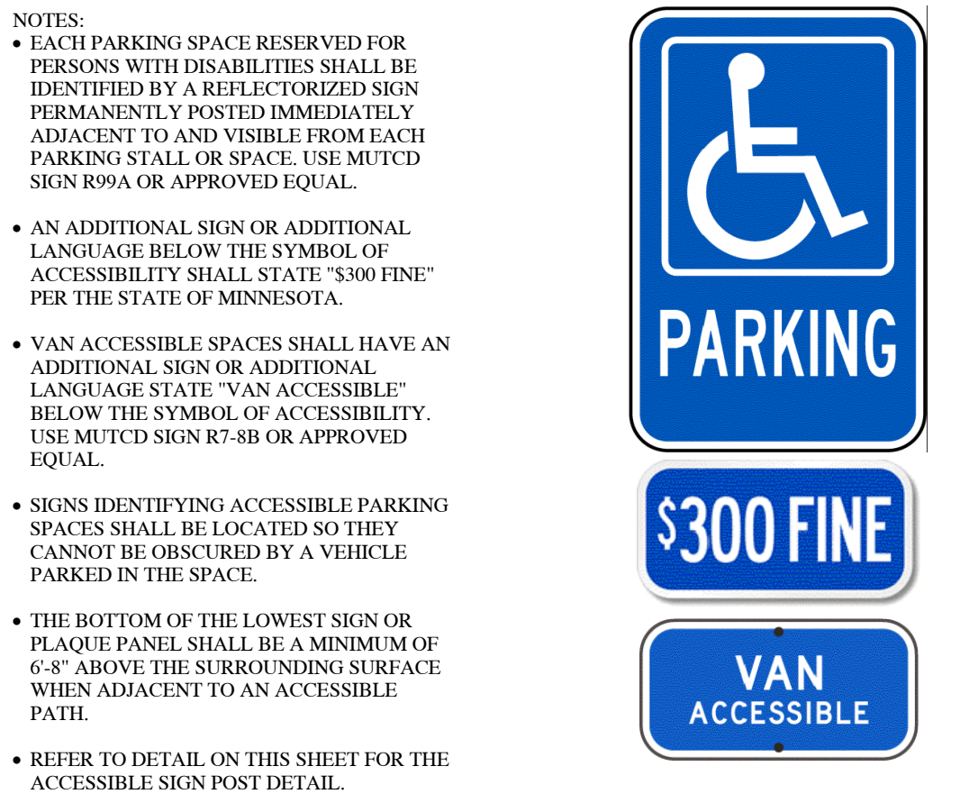
ACCESSIBLE PARKING SIGN DETAIL NOT TO SCALE
